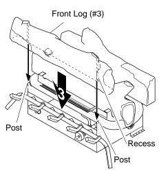
Figure 20 - Installing Front Log (#3)
